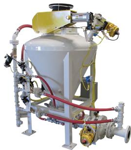
The DPP-PD Pump method discharges material with a boost by pre-pressurizing the pump full of material and then opening the discharge valve. This conveying method exploits the characteristics of fluidizable materials reducing airflow, line sizes, and power consumption.
